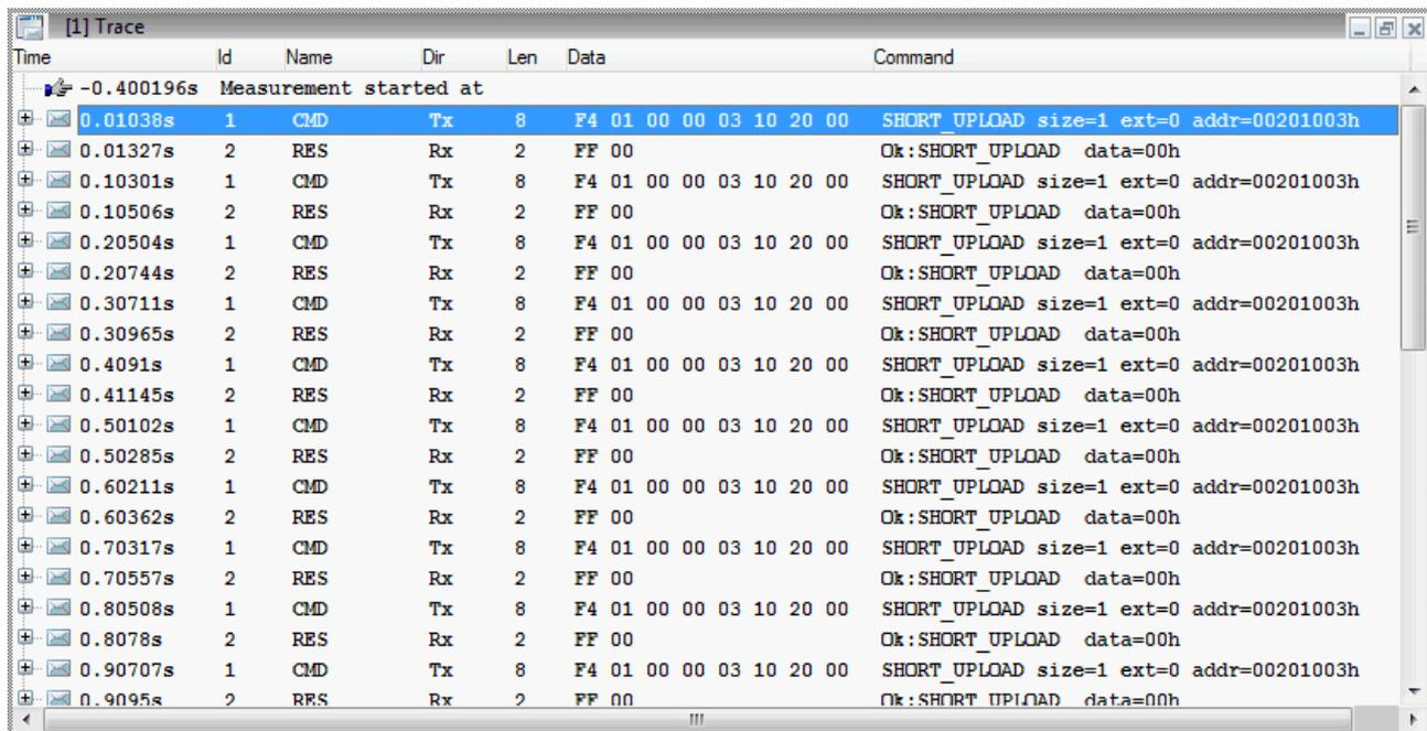
Figure 3-4: Communication sequence for the **polling** measurement mode
