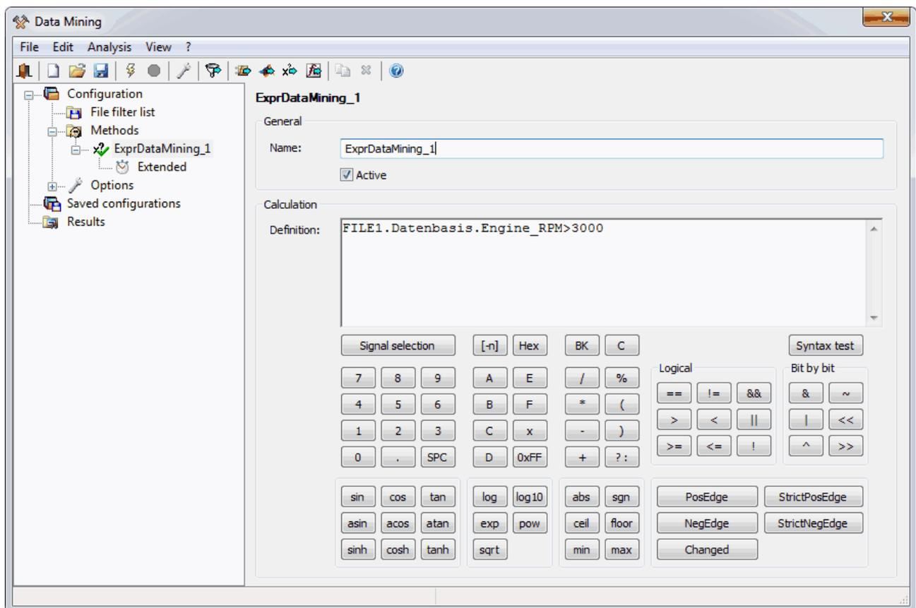
Figure 7-17: Data Mining: Creating an algebraic condition
