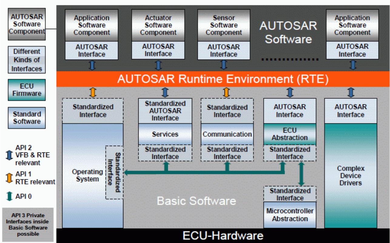
Figure 2-4: AUTOSAR software architecture<sup>2</sup>
