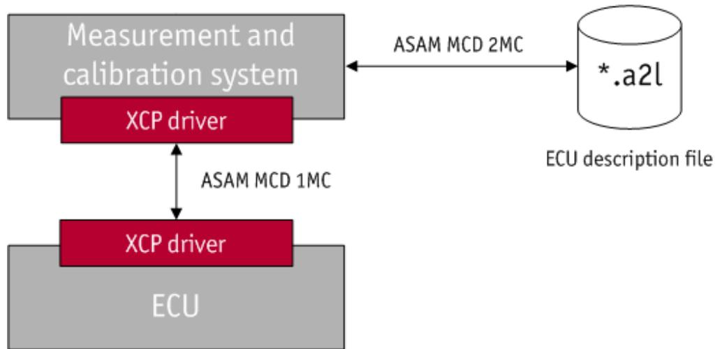
**ECU description file** The description file of the ECU for configuring the models and the layout of the calibratable and measurable objects supplies the ASAP2 (ASAM MCD 2MC) interface in the form of the A2L file. Finally, the data exchange between the MCD system and the ECU is specified via the ASAM MCD 1MC (ASAP1b) interface.
