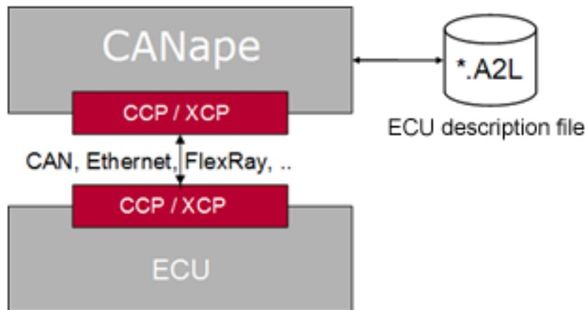
**ECU-independent concept** An ECU-independent concept for measuring and calibrating AUTOSAR applications is needed for the development of ECUs based on the AUTOSAR Standard. The AUTOSAR Calibration user manual describes a standardized procedure for implementing and calibrating an ECU according to AUTOSAR.
