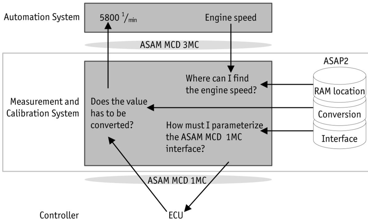
Figure 3-12: Mode of functioning of the A2L
