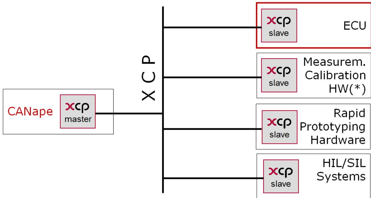
Figure 3-2: Communication possibilities of an XCP master such as **CANape**
