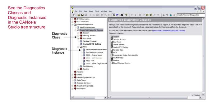
The structure within CANdela Studio is top down. In the tree on the left of CANdela Studio you will find the diagnostic class and the diagnostic instances as shown in the figure above.
