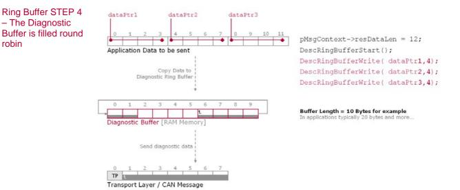
Now there are only four bytes left to be copied to the Diagnostic Buffer. The first two bytes are stored in position 8 and 9 of the buffer, the next two bytes in position 0 and 1.
