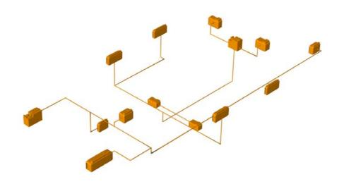
For that reason all ECUs are built-up in the same way. There is a software part to realize the main job (application) of this ECU e.g. to control the engine or a door. The other part is the software part to be able to communicate with the other ECUs via the bus system that is the communication software.
