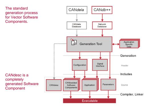
The main difference for CANdesc is that the source code for CANdesc is totally generated from the CDD file and therefore not included in your delivery as the other software components are. Since the CDD file contains most of the information about CANdesc, there are only a few configuration settings left that can be done via the generation tool on the CANdesc tab
