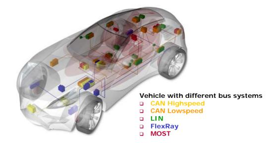
So any ECU within one bus system has to provide an identical interface to this bus system because all ECUs have to share information via this bus system as you see in the figure below.
